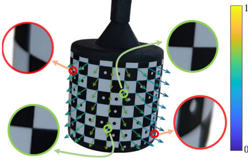
Fig. 6. Illustration of applying NVG-BA to the mouth opener. The red boxes indicate the crosspoints with severe warp, and the green boxes indicate the crosspoints with weaker warp. The vector on each crosspoint indicates its corresponding plane normal vector and the color of the vector indicates its weight.
