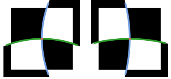
Fig. 9. Schematic diagram of subpixel corner extraction. The position of a corner is the intersection of two ellipses fitted by edges.
