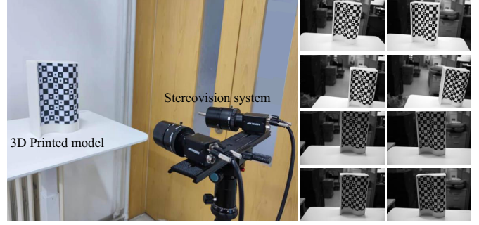
Fig. 11. Experimental setup for evaluation of the detection accuracy. A 3D printed model with a PVC marker attached on is placed in front of a stereovision system. The image pairs on the right are captured by this system.
